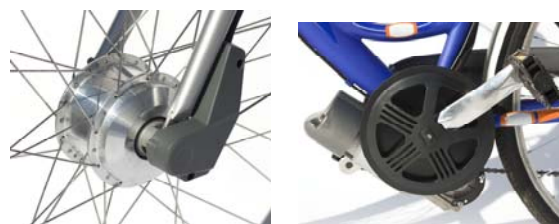
Figure 3: example of a hub motor (left) and of a motor near the bottom bracket (right)
