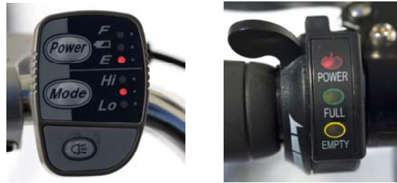
Figure 4: Selection of different assistance modes (left) and modulation of electrical assistance with a thumb switch (right)
