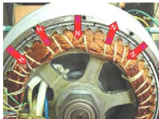
Inner view of the wheel motor with pole direction
