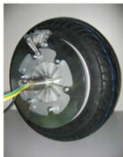
Inner view of the wheel motor with pole direction
