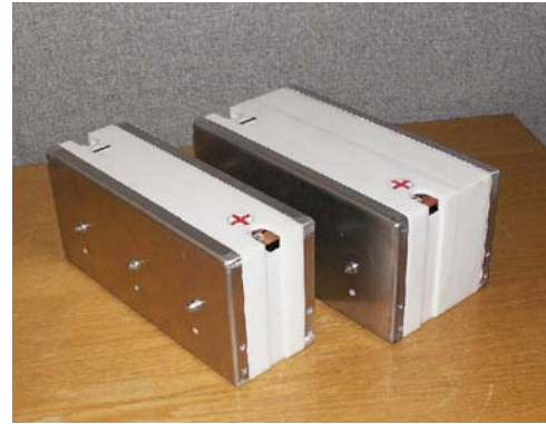
Figure 9: The engine cranking capacitor modules developed in this work.
