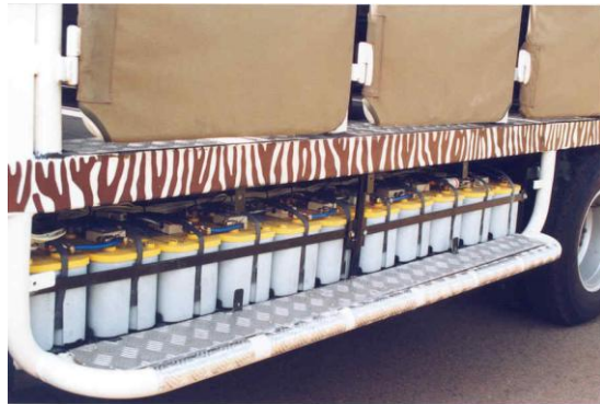
Figure 13 The Battery Compartment: Lead acid batteries were installed in the space between the front and rear wheels under the load bay.
