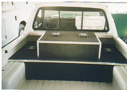
Figure 4 The battery box in the load area.
