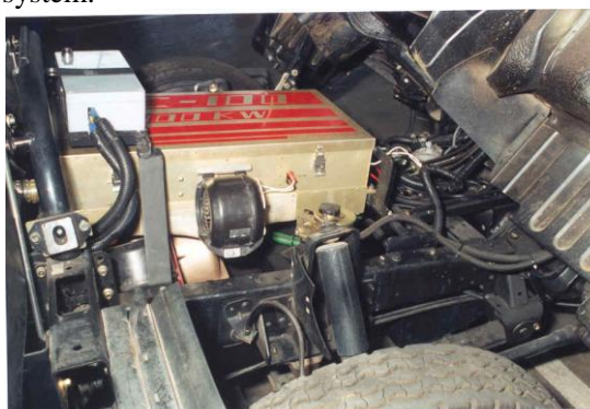
Figure 12 The engine compartment: The electric motor and controller box replaced the diesel engine.
