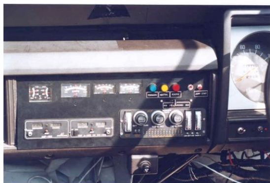
Figure 14 Monitoring and Control System for the Energy Storage System (Battery Pack).
