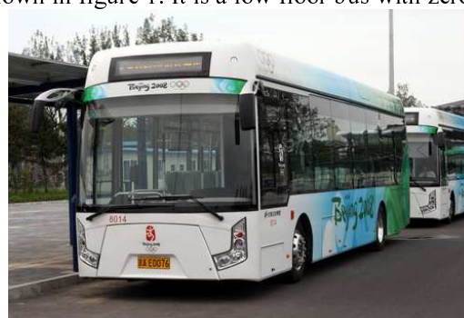
Figure 1 Olympic electric bus emissions and free pollution. By means of using new type lithium ion batteries and the dispersion rapid replacement plan, synchronous automatic plug of the power wires and the communication circuits was realized in the fast replacement process of the power battery box. Because of the integrating of alternating current (AC) motor and automated mechanical transmission (AMT), the
