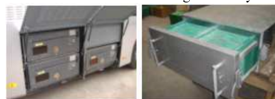
Figure 4 Structures of outer box and inner cabinet be rapid replaced with the help of machinery. The boxes are insulated suspension fixed in the vehicle to meet the needs to improve service life and reduce maintenance cost. Equipped with automatic or manual monitoring device , the battery management system (as shown in figure 5), can imply real-time accurate monitoring and
