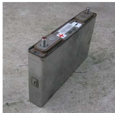
Fig. 14 Appearance of 25 Ah prototype \text{LiFePO}_4 /graphite lithium-ion cell after overcharge test.
