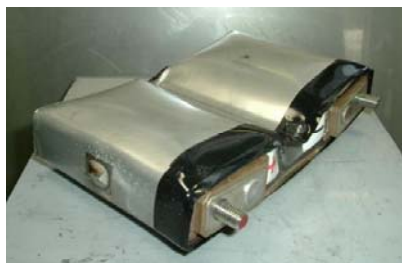
Fig. 12 Appearance of 25 Ah prototype \text{LiFePO}_4 /graphite lithium-ion cell after crush test.
