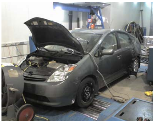
Figure 2: Hymotion Prius PHEV in Sub-Freezing Dynamometer Test Facility
