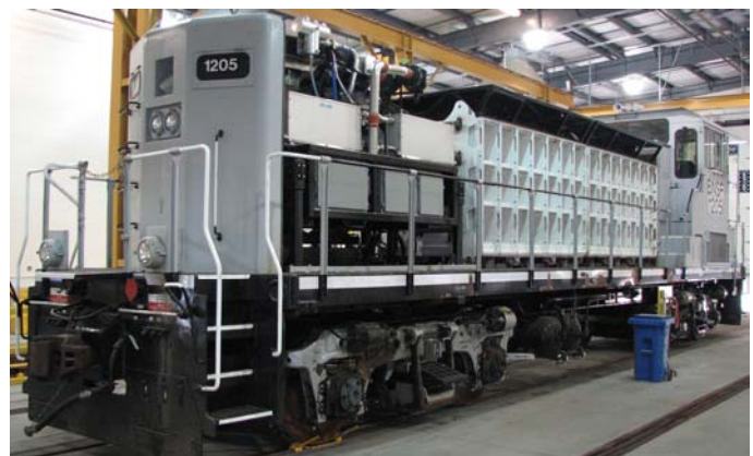
Figure 4: Right-rear view of the locomotive with the installed fuelcell prime mover in the foreground (31 July 2008)
