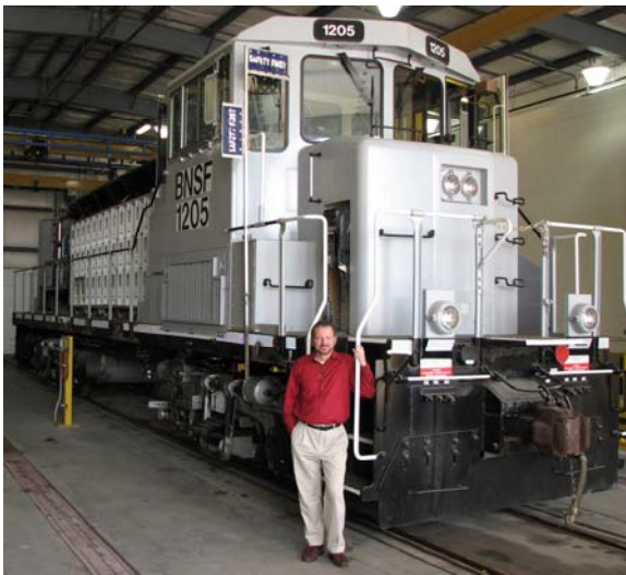
Figure 1: The fuelcell shunt locomotive, the largest fuelcell land vehicle yet built, nearing completion on 1 August 2008
