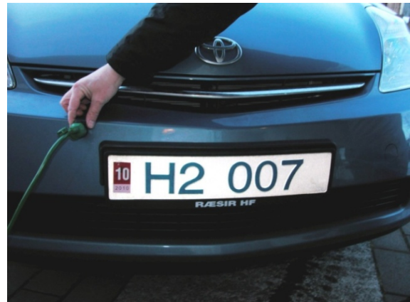
Figure 6: Connecting a block heater on Prius hydrogen car with ICE engine.
