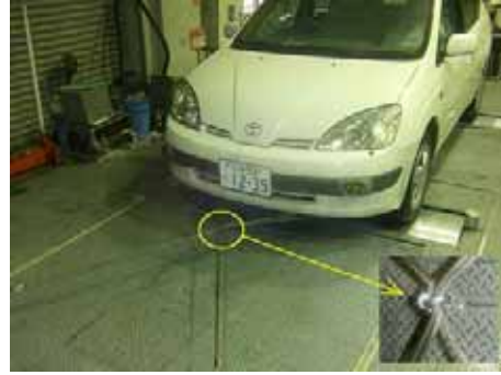
Figure 8: restraint with improved lateral stiffness
