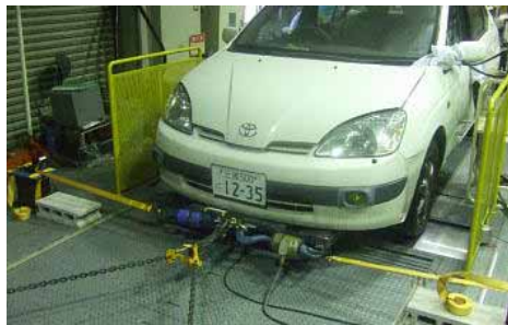
Figure 11: Rigid restraint system to find proper lateral stiffness
