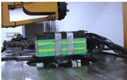
Fig.7 Vibration test of NI-MH battery
