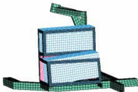
Fig.4 Deformation of frontal battery box
