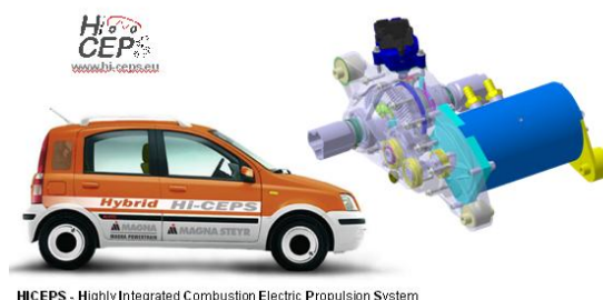
Figure 7: Hi-CEPS Panda and core electric drive module
