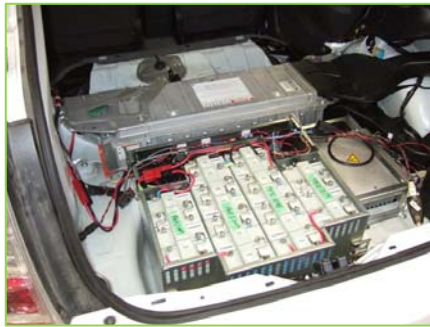
Picture 3: The NILAR battery and the in-vehicle charger.
