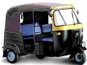
Figure 1: Three-wheeled motor taxi equipped with a 2-stroke engine [1].
