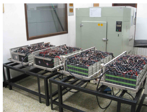
Figure 7. Ni-MH battery packs connected with test bench in laboratory
