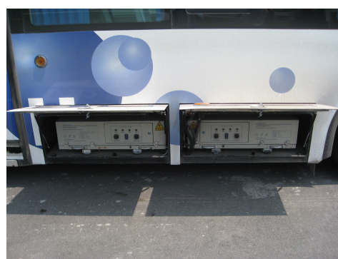
Figure 8. Ni-MH battery packs installed in Tsinghua fuel cell hybrid city bus
