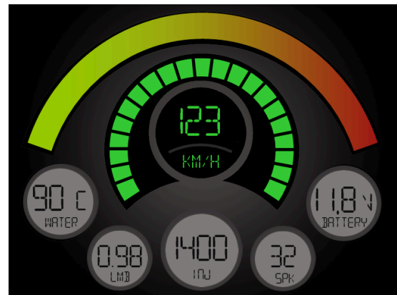
Figure 5: Digital dash board for formula SAE generated using the Dashboard module.
