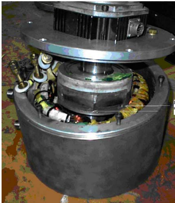
Figure 6. Damaged rotor permanent magnets.
