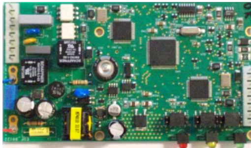
Figure 8: charging spot electronic board (74mm x 135 mm)
