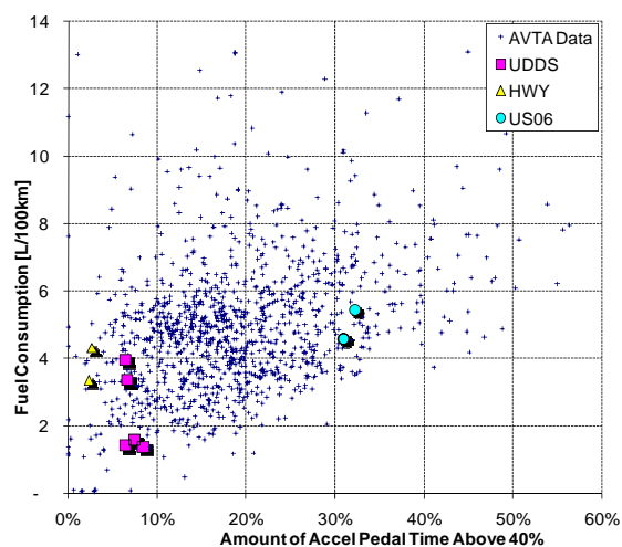
Figure 11: AVTA Fleet Time above 40% Accelerator Pedal Position versus Fuel Consumption
