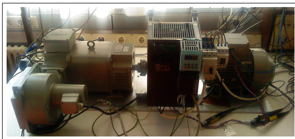
Figure 8: Back to back test-bench set-up.
