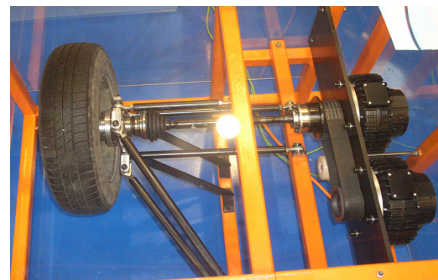
Figure 5: Detail of physical coupling between traction and mechatronic load motors.
