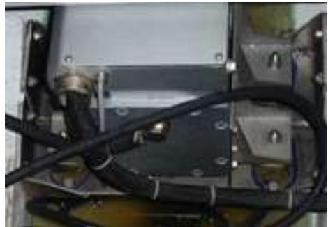
The propulsion motor is a permanent magnet motor with a nominal power of 10 kW, or approximately 14 HP. The output speed of the motor is adapted to that of the propeller without reduction unit.
