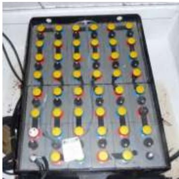
One pack of lead-acid batteries provided by SODETREL, with a capacity of 460 A.h with 48 V, produce a power of 22 kWh for a total weight of nearly 500 kg.
