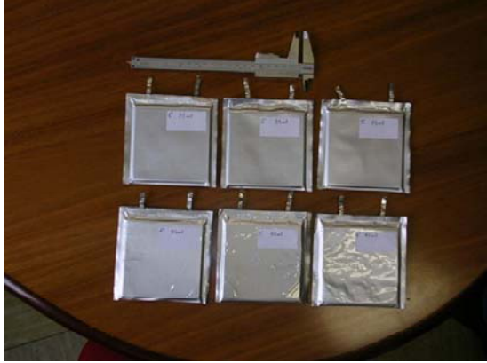
Figure 3: Carbon/IL/carbon symmetric ILHYPOS prototype cells.
