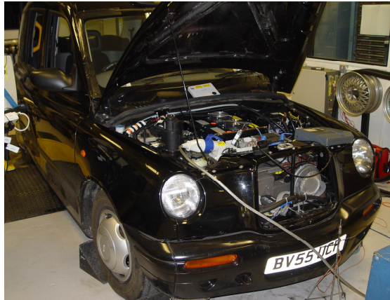
(a) Benchmark BEV, an all-electric taxi during rolling road testing.
