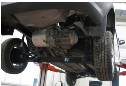
Figure 8: Electric powertrain ECO ELECTRA mounted in the rear side of the vehicle. Working on the mule vehicle
