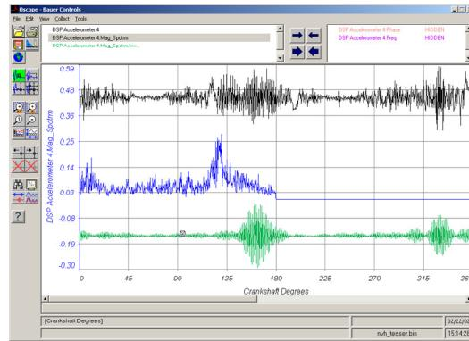
Waveforms are stored in files called recordings, which can be compressed to save disk space. Recordings are sets of data values collected at a specified rate. Recordings are linked to the related test result records for easy access.
