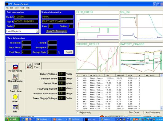
The Auto Mode window displays data in real-time as it is being collected.
