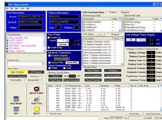
The Manual Mode window also contains controls that allow you to specify analog output values and collect data under your choice of test conditions. The window also contains a list of special functions that permit such changes as modifying solenoid settings, tuning PID loops, performing shunt calibrations, manually reading or writing to the RF tag, and setting valve configuration.
