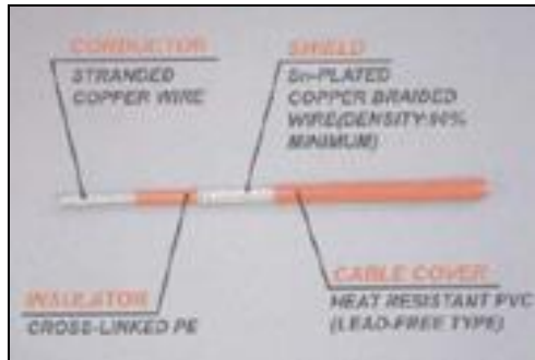
Figure 2: Structure of typical electric cable for HEV use [5]
