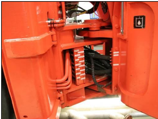
Figure 7: Hydraulic hoses in wheel loader with articulated steering (frame steering). This typically challenge both for assembly and external wear of the hoses.
