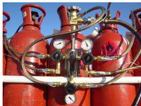
Figure 14. Portable Main flow for hydrogen filling; connected to locally standard hydrogen cylinders
