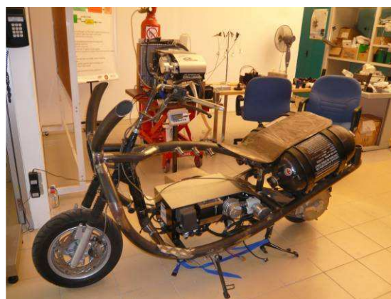
Figure 6. Custom made fuel cell motorbike frame with fuel cell system and hydrogen cylinders installed.
