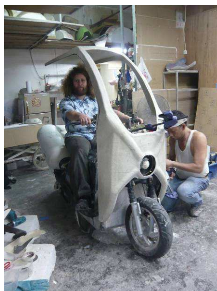
Figure 7. Bodyworks of motorbike with negative casting of Fibre glass and carbon fibber fairing parts
