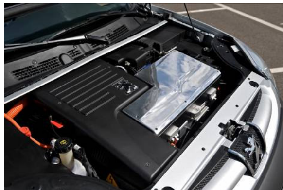
Figure 5: Fuel cell shown in vehicle engine bay
