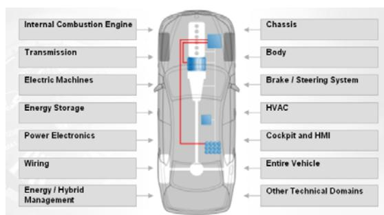
In principle all of the mentioned systems (except the internal combustion engine and possibly the transmission) must be adapted for a whole electric vehicle, too. So it needs a system approach and an interdisciplinary cooperation of body & white designers, crash, chassis (due to the high load) and electric and electronic experts to find practical solutions for the overall system changes. Some of these approaches, successfully used in several projects, are:
