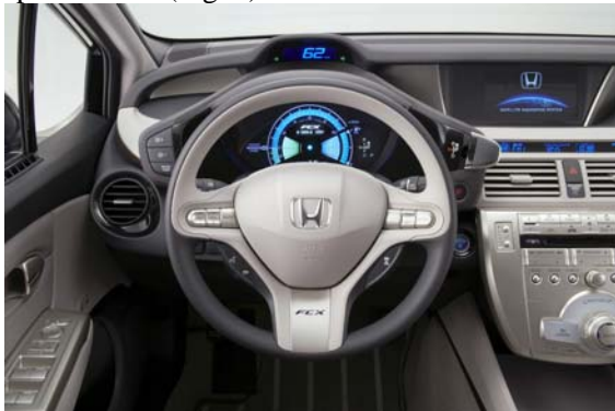
Figure2: FCX multiplex meters (multi-layered instrument panel)
