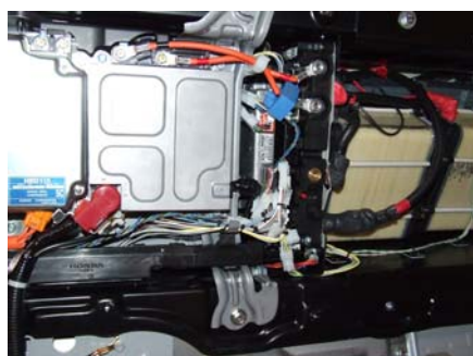
Figure 16: The Effpower bipolar battery (right) in the Civic
