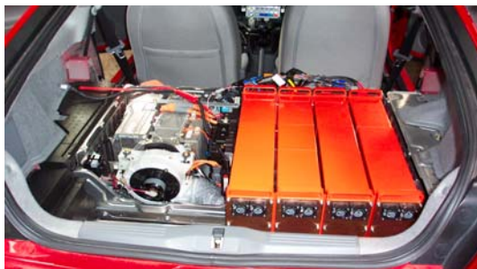
Figure 1: Rholab modules in the vehicle
