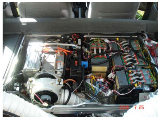
Figure 2: Effpower battery in place
