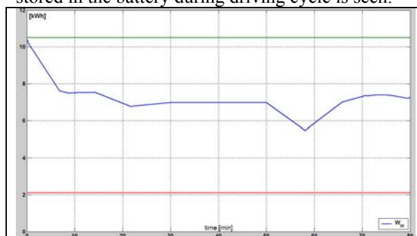
Figure 6. Time dependence of the energy stored in the battery during driving cycle. Upper and lower lines represent energy limits of the battery.
