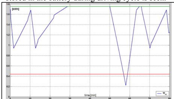
Figure 8. Time dependence of energy stored in the super capacitor during driving cycle. Upper (green) and lower (red) lines represent energy limits in the super capacitor. It is seen that under given driving cycle it is not possible to carry out the desirable driving cycle in silent interval. As it is seen from the graph, 75% of the SC energy is not sufficient for desirable driving regime. It is necessary to start ICE at 57 th minute of driving cycle.
