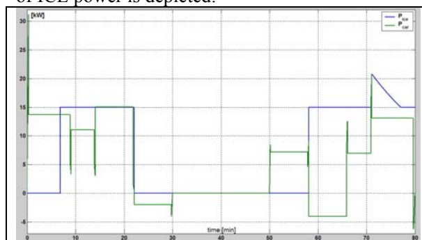
Figure 5. Time dependence of vehicle power demands during driving cycle. Blue line – ICE power, green line- power on driving wheels needed for vehicle movement
