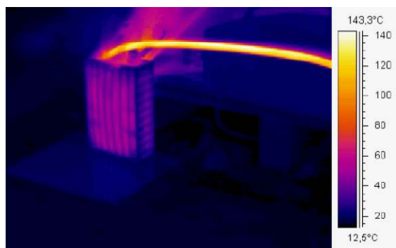
Figure 9: Thermal camera picture of cell venting.
