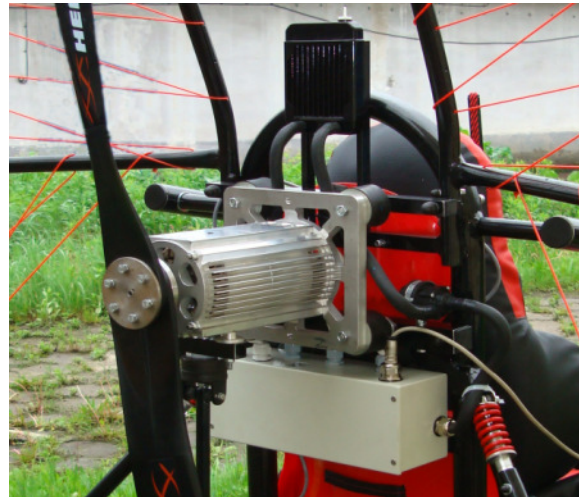
Figure4: The frame of electric motor mounted in paraglider
