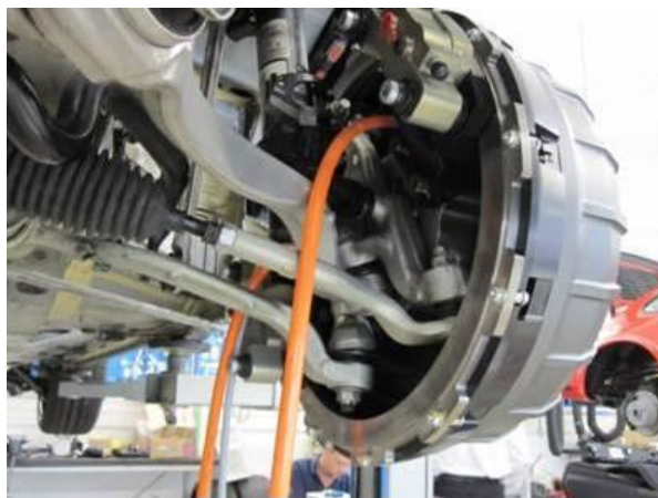
Figure 8: Left motor and brake assembly
