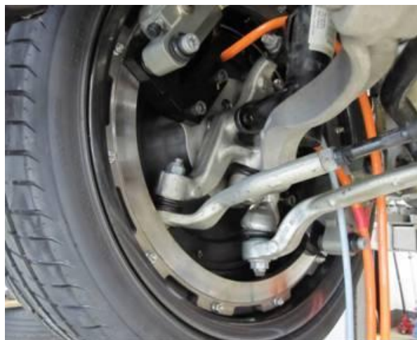
Figure 9: Right motor and brake assembly with wheel
