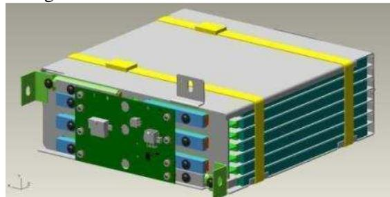
The blocks was placed in specially designed “cage” designed to meet space and durability requirements. Example of mechanical structure for modules is shown below:
