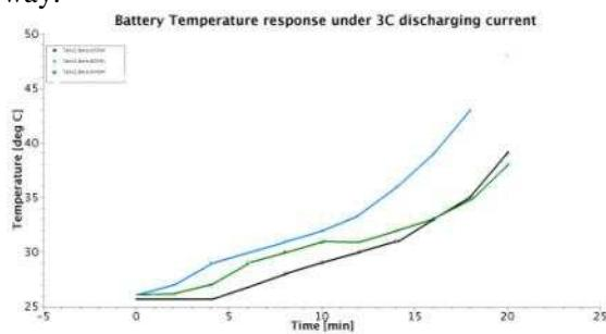
This effect results with limiting performance of the sport car and is also dangerous due to possible thermal runaway of whole battery pack.
