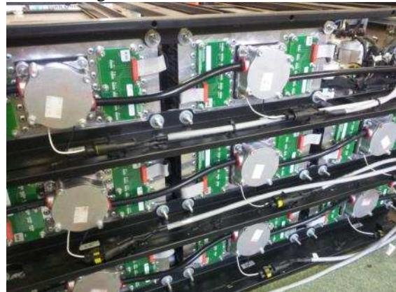
Peltier modules are controlled by dedicated power drivers which are connected to dBGS for gathering information about thermal management strategy. By controlling the current of the Peltiers modules system can very precisely manage the temperature of cells.
