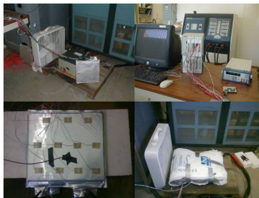
Figure 2: Testing of the 50 Ah lithium titanate oxide cell
