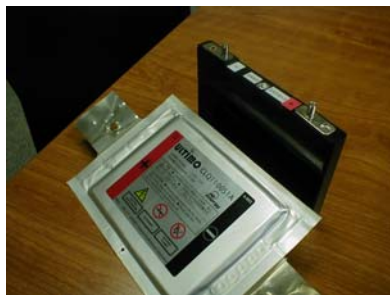
Figure 1: Photographs of the JM Energy 1100F and 2300F devices
