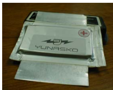
Figure 2: Yunasko Hybrid ultracapacitor 5000F device
