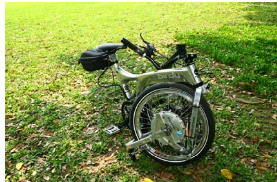
Fig. 2. The foldable e-bike
