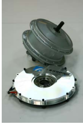
Fig. 4. The traditional motor and the slim motor
