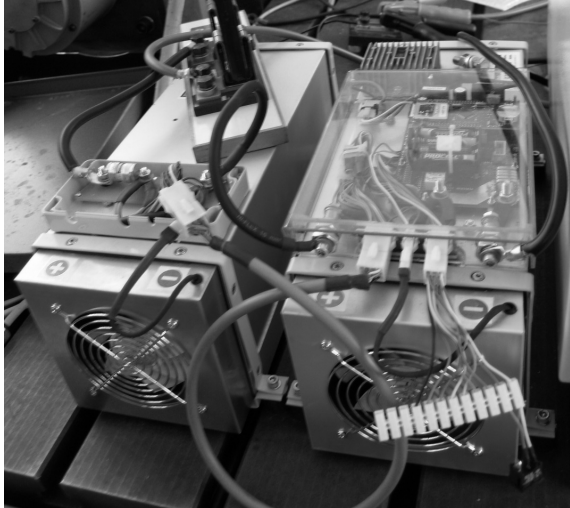
Figure 3: The lithium iron phosphate battery of the high voltage power net.
