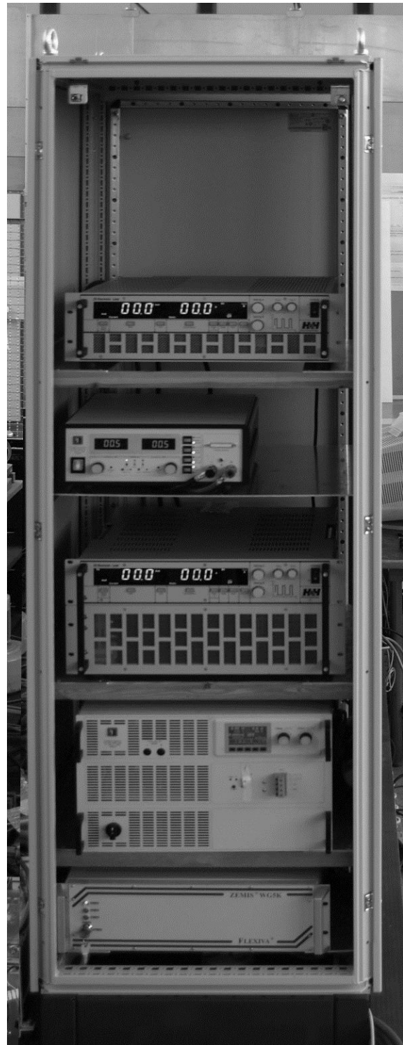
Figure 2: The components of the second voltage level test bench that are built in a test bench. The battery is separately placed, see Fig. 3.
