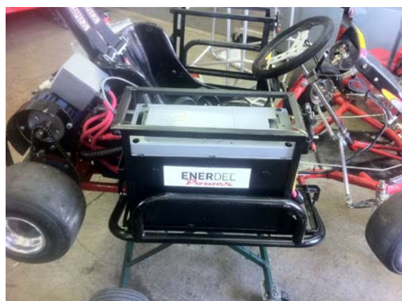
Figure9. The Battery exchange system
