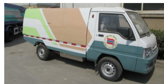
c) 2-ton electric garbage collection vehicle
