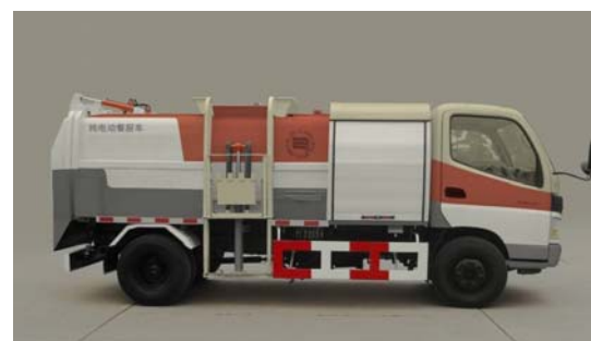
b) 8-ton electric cook garbage collection vehicle
