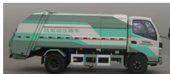
a) 16-ton electric garbage vehicle
