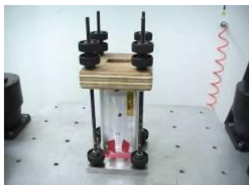
Fig. 14 Mechanical shock test (UN38.3)
