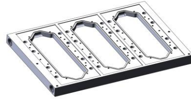
Figure 4: The structure of the driver's cooling base (IGBT discrete I)
