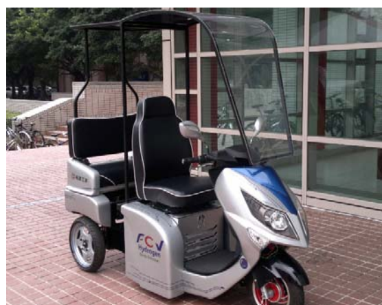
Fig.9 Tourist LEV of hybrid power system with fuel cells as range extender
