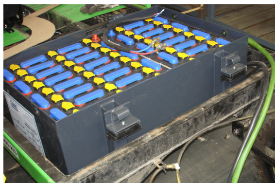
Figure3: Lead-acid battery pack used in electric platform tractors, nominal battery voltage 80 V
