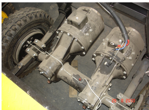
Figure2: Two DC series motors installed in one of the old solutions of electric drive for battery-powered electric platform tractor manufactured in Poland
