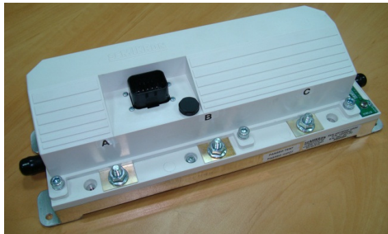
Figure5: Inverter type SKAI 4201MD20 (Semikron) with 200 V MOSFETs
