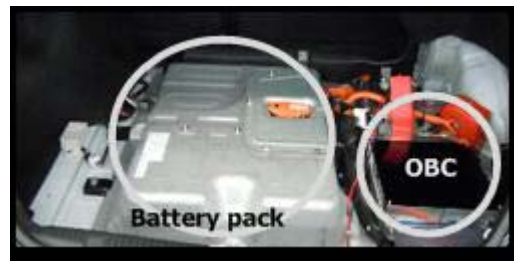
Figure 10. Battery pack & OBC in HMC EREV
