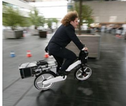
Figure 1. The first author with fuel cell electric bicycle prototype with 250km range and a total weight of 26kg in Hannover Messe 2010
