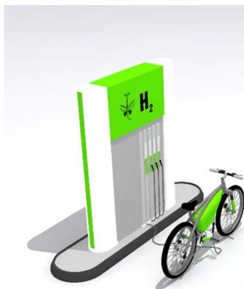
Figure 4. Monarch Bicycle equipped with integrated fuel cell power pack at hydrogen refueling station
