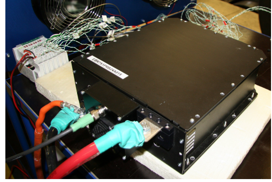
Figure 5: Battery under test. Additional temperature sensors have been attached inside the module.
